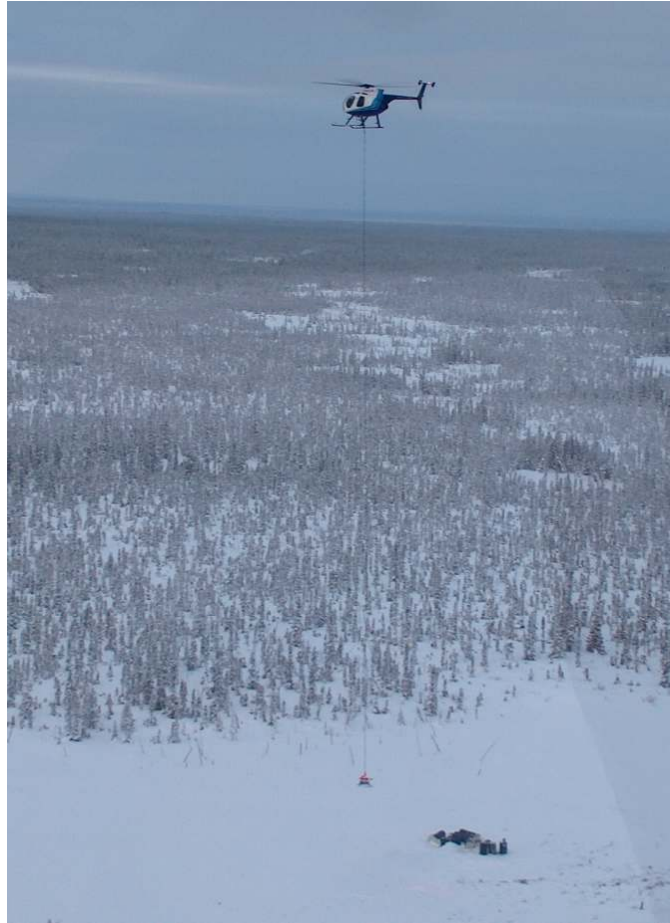
Figure 4. Hughes 500 helicopter and longline gravity meter on the 150 foot longline
